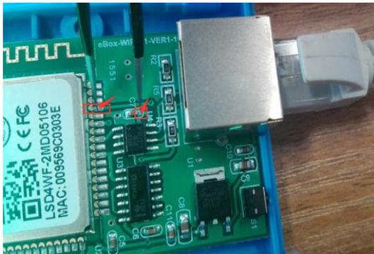
If the link light flash once (As follow figure ③), the WiFi module restores successfully, then release the tweezers.
